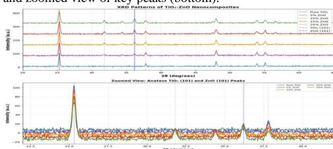
Figure 3: XRD patterns of TiO 2 -ZnO nanocomposites (top) and zoomed view of key peaks (bottom).
