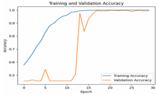
Figure 7: Accuracy Graph for Training and Validation of CNN.
